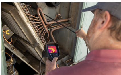
VSC-IR21 Probe 19 mm round forward viewing tip
