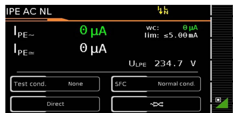
Test sequence – IPE Measurement (IEC 62368/EN 62368/VDE 0868-1)
