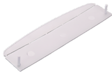
33155 000 barrier for handle for NH fuse-switch disconnecter size 1-3 for closing of handle area from rear
